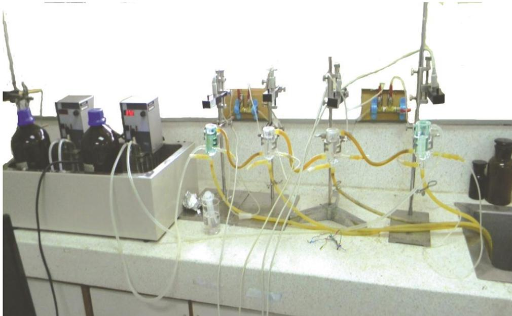
Figure 1: Set up for isolated organ bath. [Heto Lab Equipment BIOPAC System (water bath), Scientific Promotion Co. Ltd., Model MP 100 1759 Soiwachirathumsathit, 11 Sukhumvit, 101/1 Bangkok, Prakanong, Bangkok 10260; Programme – Labscribe 2 – iWOR x 1, Washington Street, DOVER NH 03820]
